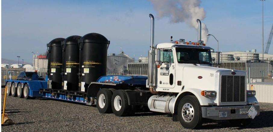
First waste containers awaiting disposal at Hanford's Integrated Disposal Facility (vitrified waste cannisters then put into disposal vessels).
